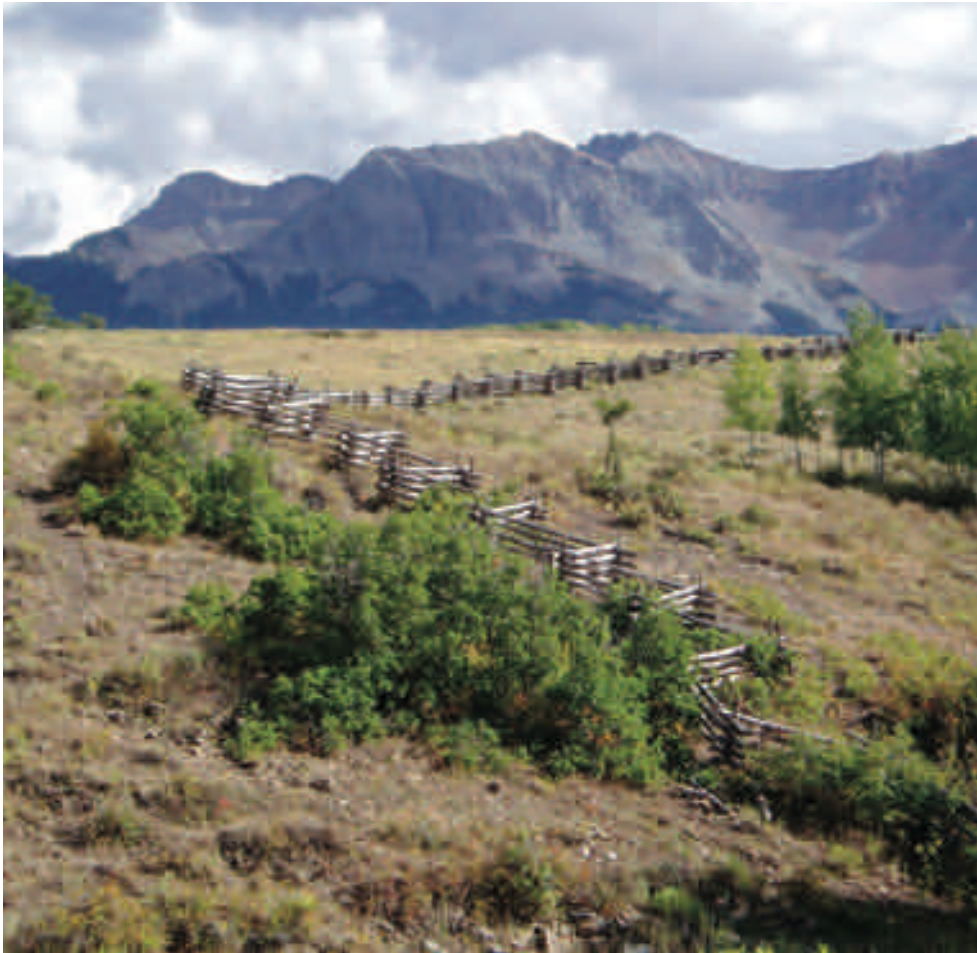
Worm or zig-zag fence is often used on rocky or uneven ground.
